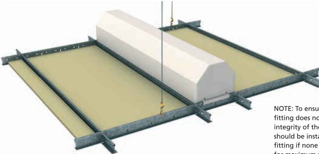
■ FIGURE 7: LIGHT FITTING DETAIL
