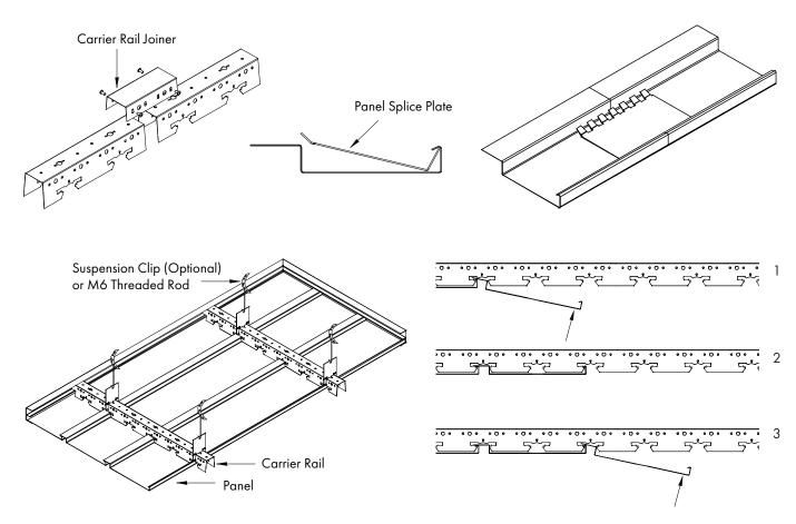
METALWORKS F-Plank are simply raised into position and clicked into the Carrier Rail. Refer to the METALWORKS F-Plank System Components and also the Assembly and Installation Instructions for more details.
